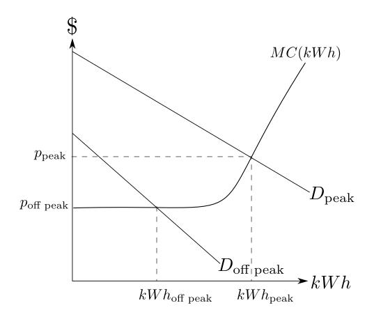
Currently, a regulator mandates that the electric company set price equal to marginal cost in both the peak and off peak markets, leading to the current peak and off peak prices of  $p_{\text{peak}}$  and  $p_{\text{off peak}}$  shown on the graph as well as the corresponding quantities  $kWh_{\text{peak}}$  and  $kWh_{\text{off peak}}$ .
